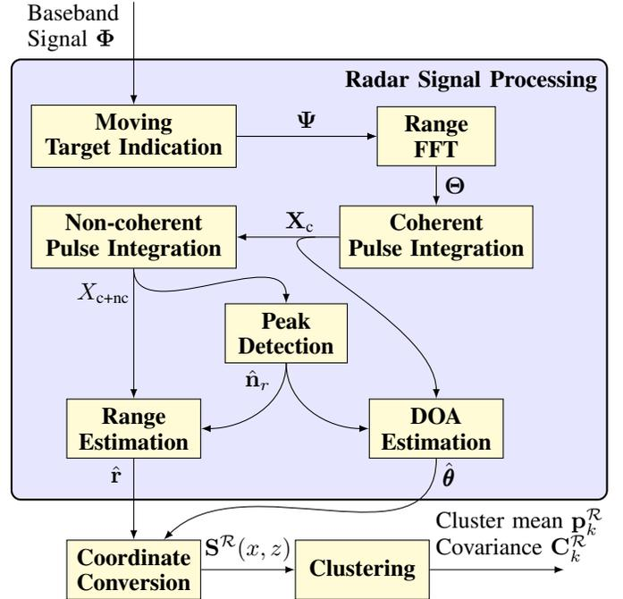
Fig. 4. Overview of the radar signal processing chain.
