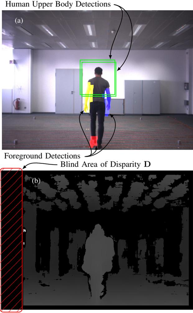
Fig. 3. (a) Results of upper body and moving foreground object detection from the left camera image. (b) Disparity map estimated from the left and right image.
