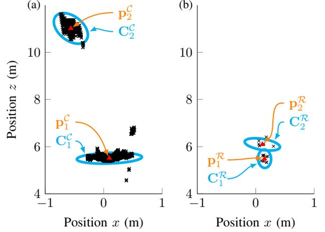
Fig. 6. Detected targets for the scenario in Fig. 3(a). (a) From image. (b) From radar signal.
