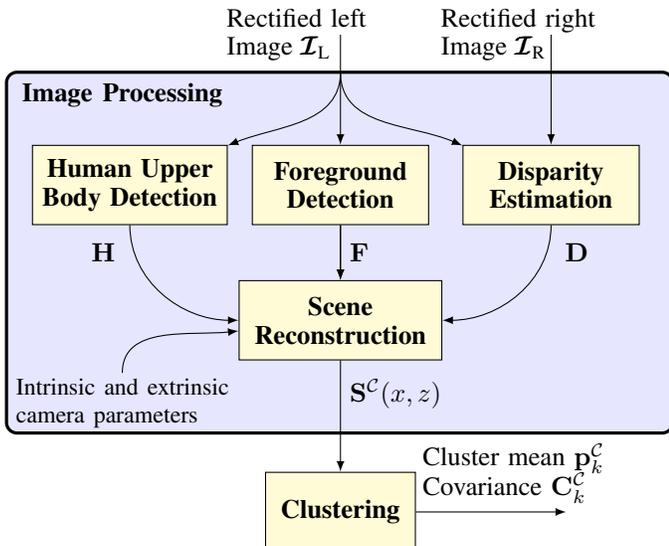
Fig. 2. Overview of the image processing chain.
