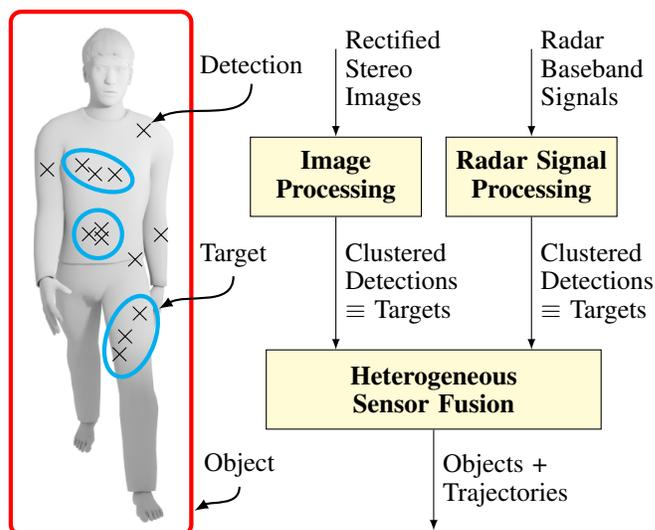
Fig. 1. Overview of the fusion system for indoor detection and tracking of pedestrians.
