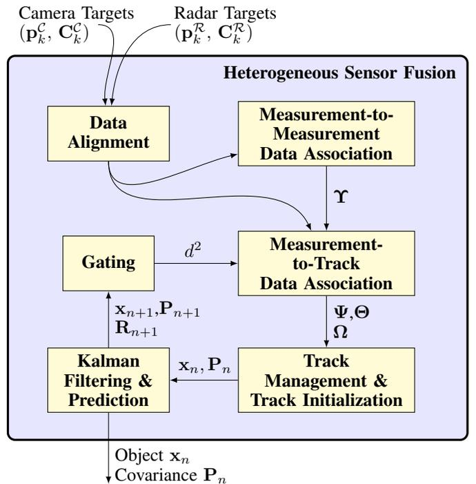
Fig. 7. Overview of the heterogeneous sensor fusion chain.
