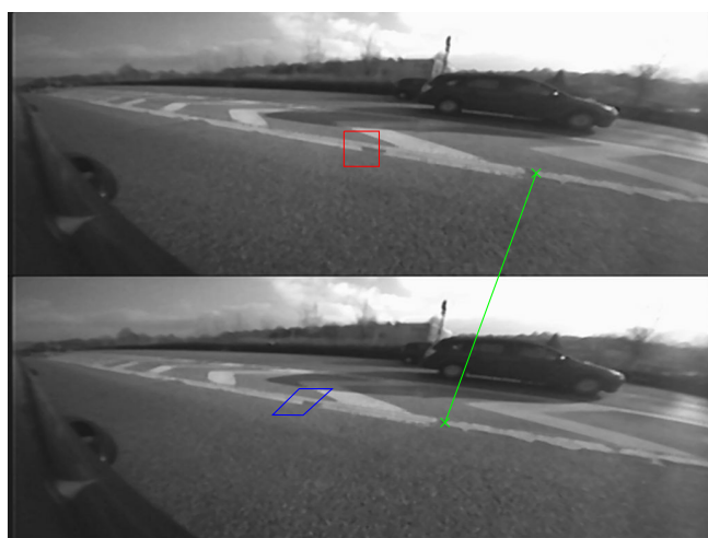
Fig. 2. Two consecutive frames of a video sequence with one exemplary feature pair (green line) and a rectangular region of size 32x32 (red) in the top image and the equivalent transformed region (blue) in the bottom image
