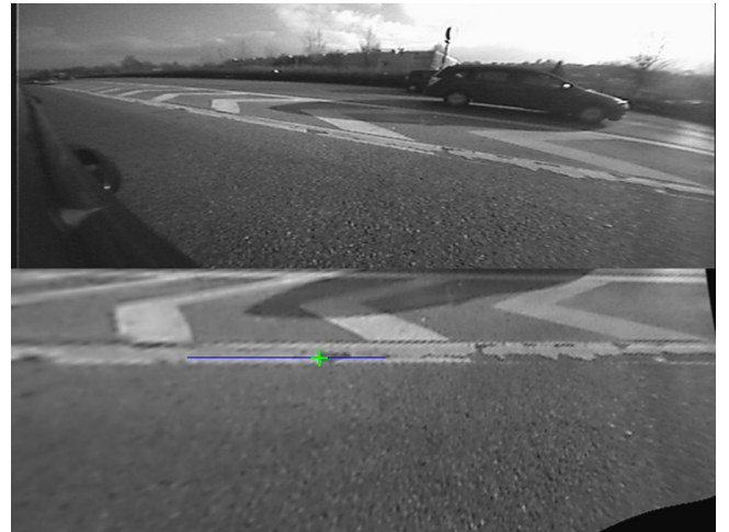
Fig. 5. The original and the transformed version of an image, one exemplary feature point extracted on the road surface (green cross), the horizontally aligned scan line for the disparity estimation (blue line)
