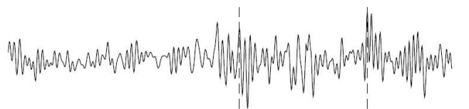
Fig. 2. GCC-PHAT of two microphone signals for two speakers in a room
