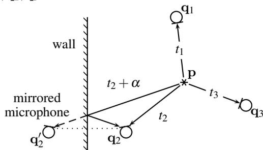
**Figure 5:** Change of the distance between one microphone and the source as caused by echo path propagation or mirrored microphone
