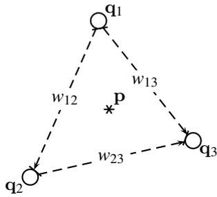
**Figure 3:** Initial scenario for TDOA based localization
