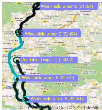
Figure 3. Windshield wiper lever position on the route for rain and snow detection
