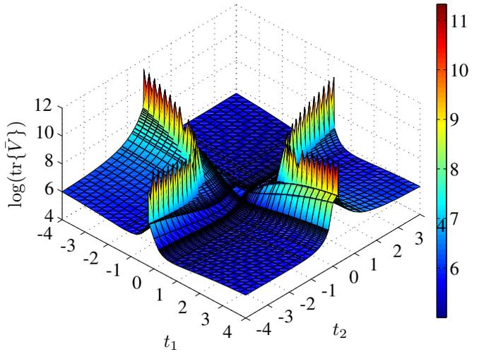
Fig. 4. Upper bound  $\text{tr}\{\bar{V}\}$  of the expected estimation error over the precoding matrix  $T$  for Example 1
